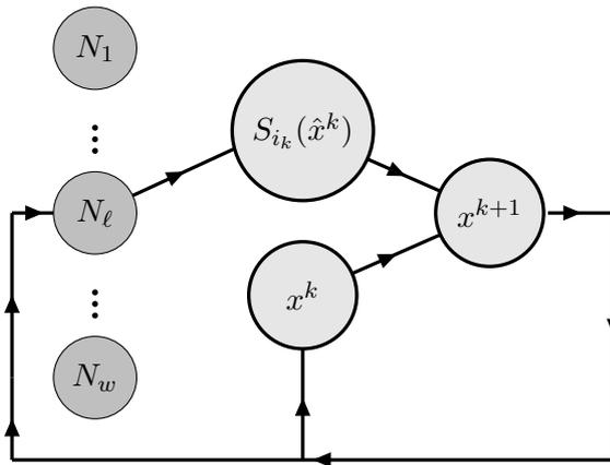
Fig. 2: Schematic architecture for the ASI algorithm. At the current iteration  $k$  the latest output  $N_\ell$ , which is precisely  $S_{i_k}(\hat{x}^k)$  in the ASI algorithm, from the  $\ell$ -th node is merged with  $x^k$  via a linear combination to form the update  $x^{k+1}$ , overwriting the global variable  $x^k$ . Here  $w \leq m$  is the number of processing nodes.
